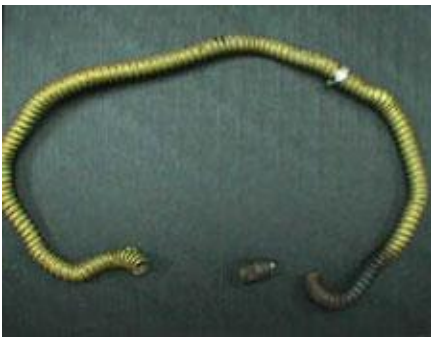
↑ Uncoated brass connector BAD – DO NOT USE
